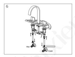
G. Apply Teflon (TPFE) plumbing tape on both valve assemblies and shutoff valves. Attach water supply hoses with 1/2" fittings (not included) with an adjustable wrench. Also connect the water hose between the handle assemblies and the center spout. (NOTE: Do not overtighten the connection.)
