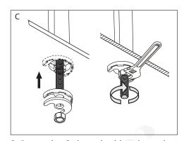
C. Insert the C shaped rubber / metal washer and locking nut on the center spout. Use an adjustable wrench to secure spout in place. (NOTE: Do not over tighten the locking nut.)
