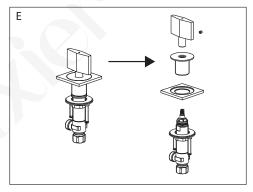
E. Use a small hex wrench to loosen the small setscrew on the handle. Lift up the decorative trim handle and remove all trim pieces.
